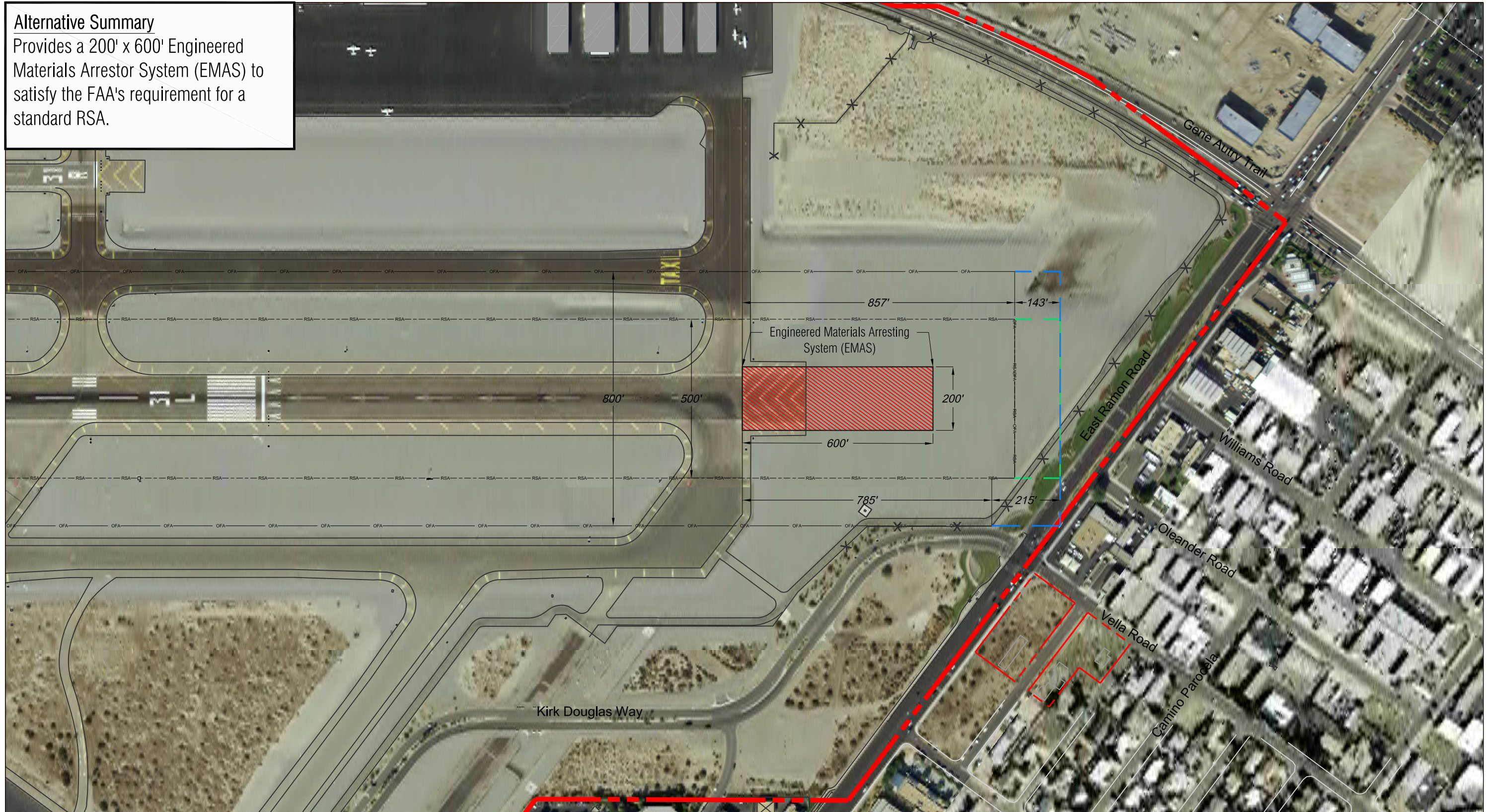
Alternative 1 - Runway Safety Area - EMAS Figure 5-2 Palm Springs International Airport Master Plan
