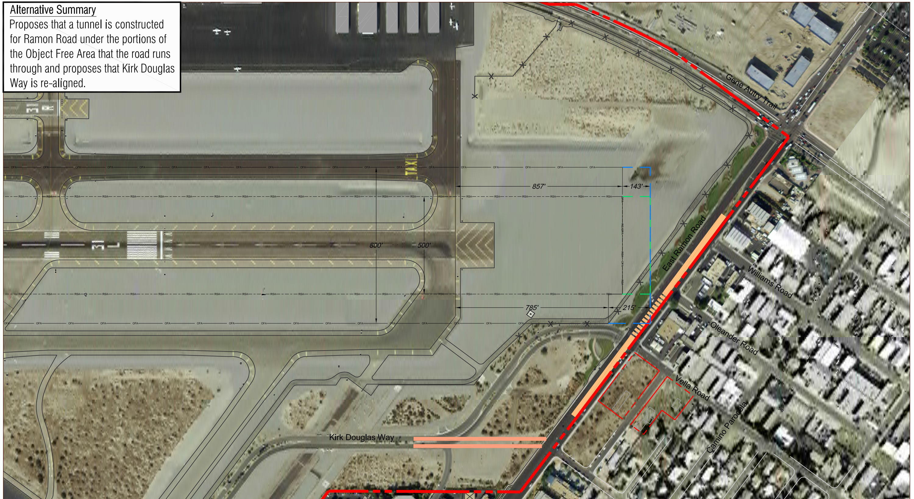
Alternative 2 - Runway Safety Area - Tunnel Figure 5-3 Palm Springs International Airport Master Plan
